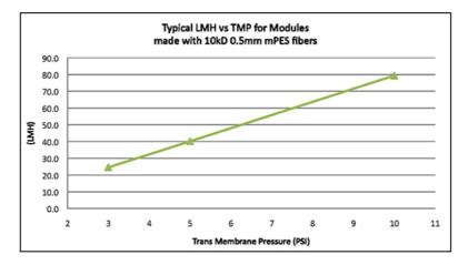
Figure 11. Typical LMH versus TMP for modules made with 10 kD 1 mm mPES fibers
