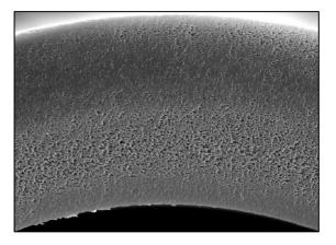
30 kD 0.5 mm ID Spectrum<sup>®</sup> mPES Hollow Fiber @ 750X magnification
