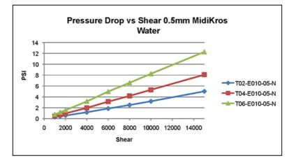
Figure 23. Pressure drop versus shear 0.5 mm MidiKros TC 25% glycerin solution (15cP)
