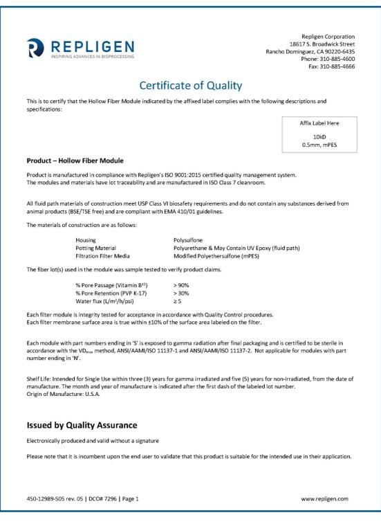
\* CoQ example is for a 10 kD 0.5 mm Spectrum<sup>®</sup> mPES Hollow Fiber Filter Module.
