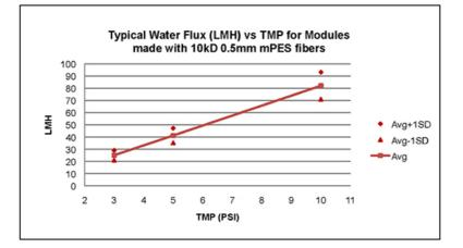
Figure 15. Typical LMH versus TMP for modules made with 10 kD 1 mm mPES fibers
