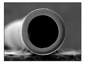
30 kD 0.5 mm ID Spectrum<sup>®</sup> mPES Hollow Fiber @ 100X magnification
